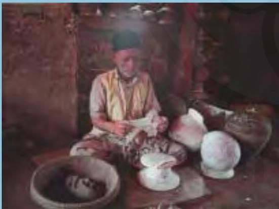
2. After the pulp is ready, clay, wooden or brass moulds are used to give it the required shape. When the pulp is dry the shape is cut away from the mould in two halves with a fine saw and glued together again.
