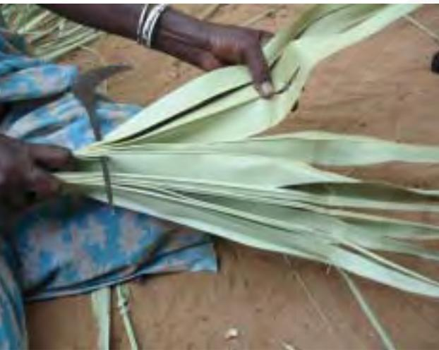
*An artisan making strips of the palm leaf by inserting a knife in the leaf fold and separating the leaf from the midrib*
