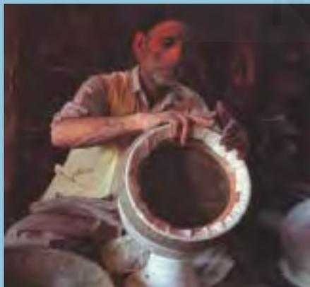
3. The surface is coated with a white layer of gypsum and glue and rubbed smooth with a stone or a piece of baked brick, called *Kurket*.
